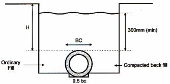
Generally only suitable for pipes up to 300mm (12in) diameter in uniform fine-grained soils where conditions are relatively dry.
