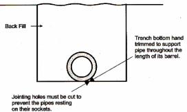
Only suitable for pipes up to 300mm (12in) diameter in uniform fine-grained soils where conditions are relatively dry. Regarding 'wide trench' loads.
